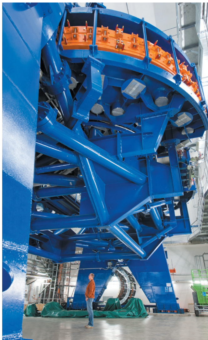
Gantries to direct charged-particle beams weigh as much as 600 tonnes.
