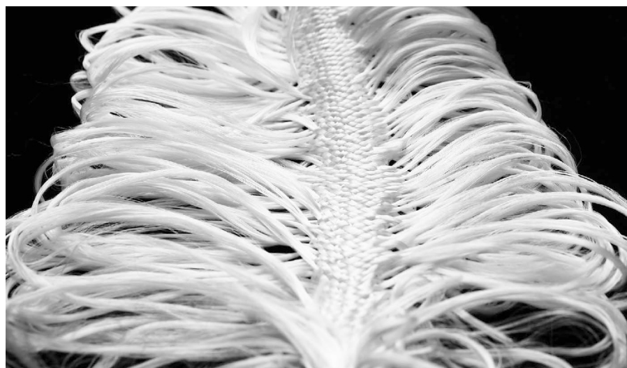
High-capacity (HiCap) polymers can separate metals such as uranium from solution.
