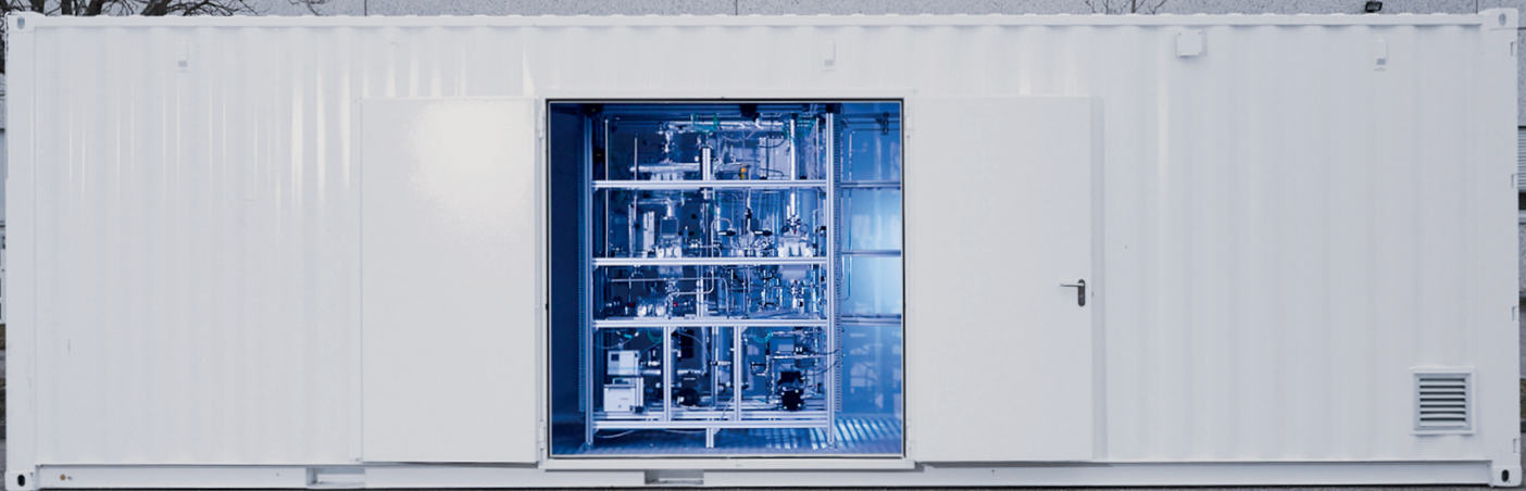
Ineratec build compact chemical reactors that fit into shipping containers.
