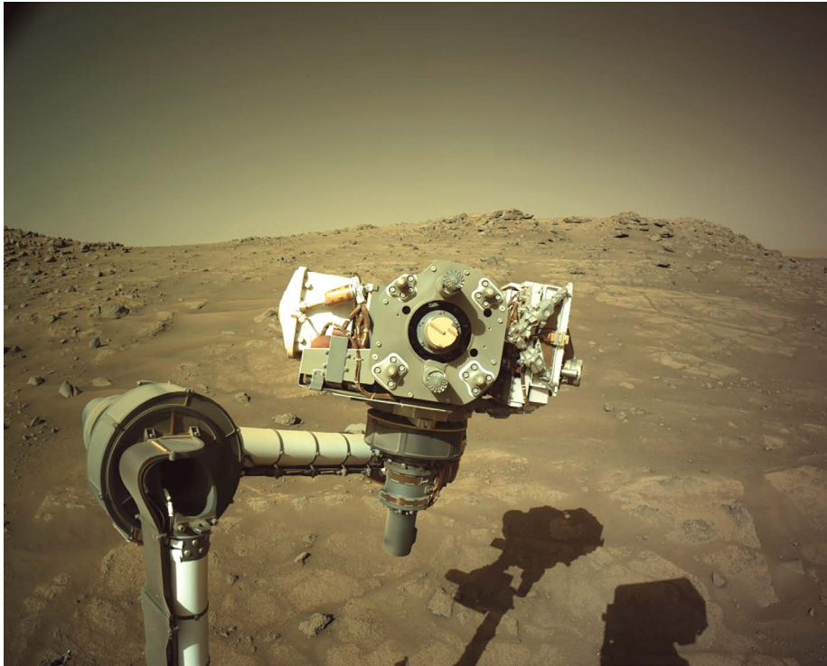
Perseverance uses its sampling arm to collect rocks and explore the planet's geochemistry.
