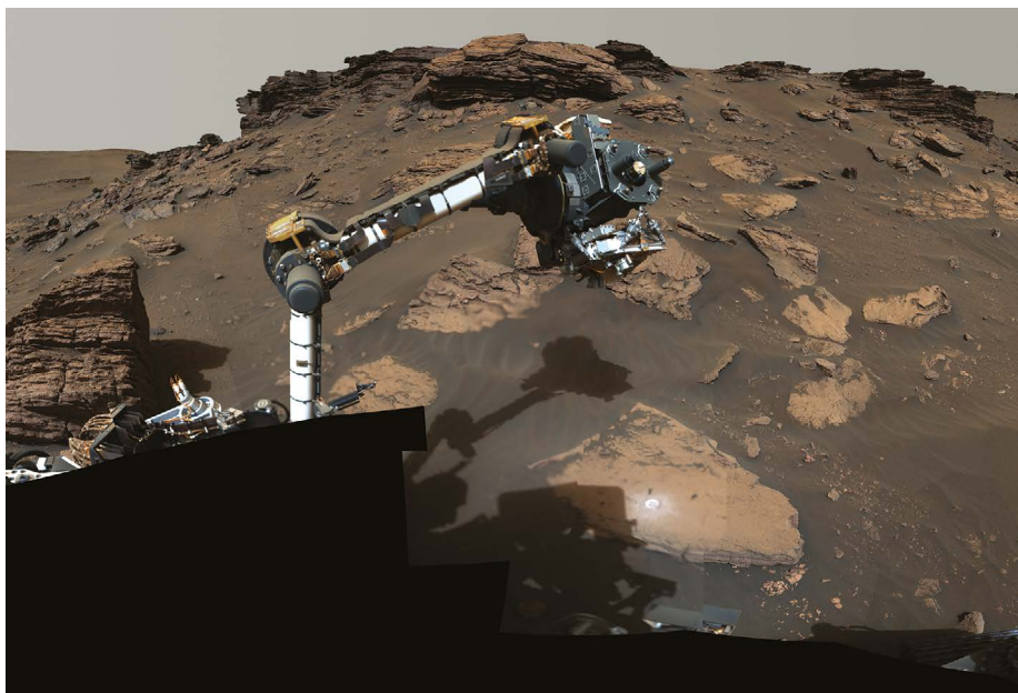
Perseverance used its robotic arm to collect rock cores from an outcrop called Skinner Ridge, which is part of an ancient river delta on Mars.
