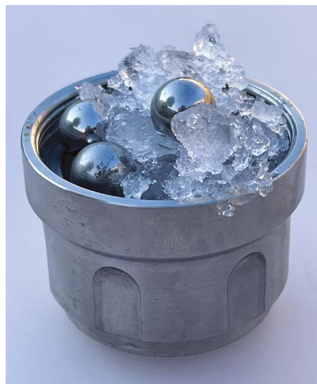
Milling ordinary ice with steel balls produced a new version of solid water.
