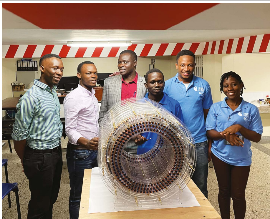
Johnes Obungoloch (centre) and his team with a magnet used in a low-field MRI scanner.
