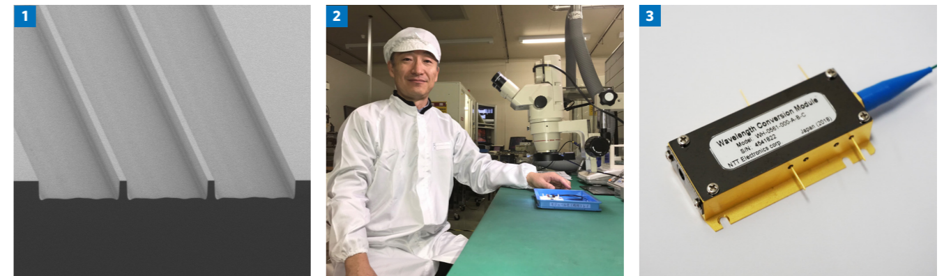
▲ 1. Electron microscopy image showing the cross section of a waveguide based on PPLN. 2. Yoshiki Nishida and his team have greatly boosted the efficiency of PPLN crystals, making them useful for practical applications. 3. A module that converts the wavelength of light using a non-linear process known as second-harmonic generation.
